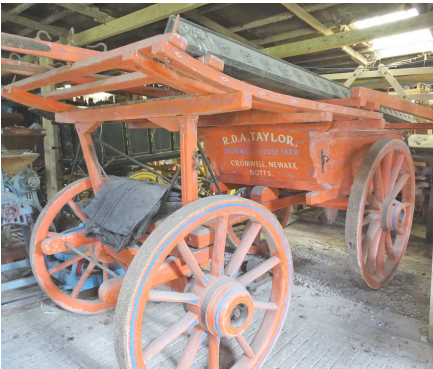
A tip cart able to take some muck out to the field as well as extend for more space for carting hay
