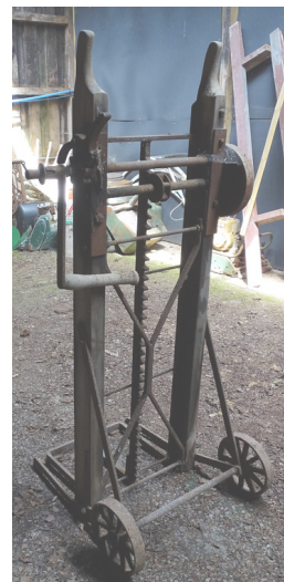
A sack hoist (not a sack barrow) for elevating sacks to the correct height so that the men did not need to bend down
